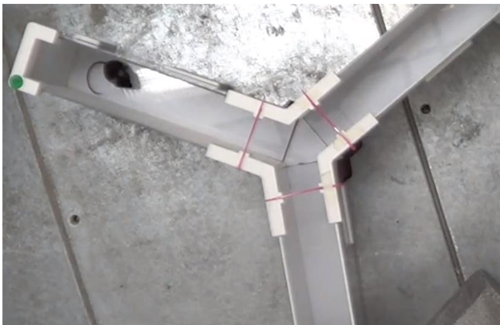
Figure 2. Y-maze was made from clear acrylic, cut with a computer numerical control router, and polyactic acid 3D printed components.
